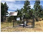
Solar-Powered Air Quality Monitor Installed at Oregon
